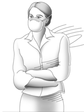
Air-purifying respirator, which removes contaminants from the air Half mask Filtering Facepiece; Dust mask Needs to be fit tested APF=10
