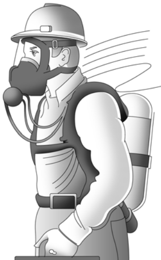
Tight-fitting Self-Contained Breathing Apparatus (SCBA) pressure-demand mode APF=10,000 Demand mode APF=50 Needs to be fit tested
