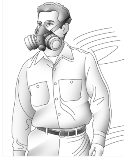
Half mask Elastomeric Respirator APF=10 Needs to be fit tested
